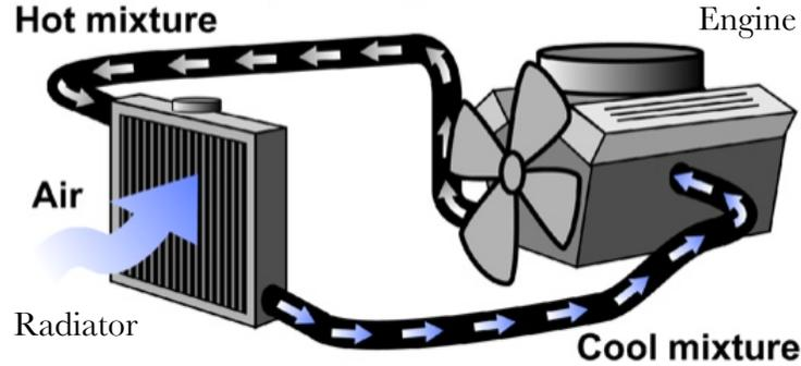
6. The figure above show the movement of a liquid in a car from the engine through the radiator and back to the engine. The purpose of this is to \_\_\_\_\_.
